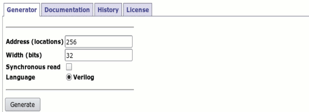
Figure 4-1 Single Port FF memory generator GUI
